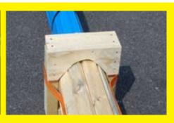
Spar-Protect is made from strips of hardboard that are sandwiched between sheets of specialist plastic to form a product that can be wrapped around spars. This, combined with a carefully designed 'bubble-wrap', and reinforced strengthening around lifting points, creates the best possible protection for spars in transit. The new system has been thoroughly tested and is currently being used for spars in transit. Initial reports are very positive:
